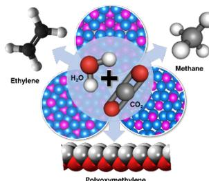
Transition metal phosphides catalyze the reduction of CO<sub>2</sub> to gaseous C<sub>1</sub>, C<sub>2</sub> hydrocarbons and solid [CH<sub>2</sub>O]<sub>n</sub> with no (toxic) CO formation. They use lower electrical potential than state of the art catalysts (Cu, SnO<sub>2</sub>, In<sub>2</sub>O<sub>3</sub>) and require no process heat or pressure (ambient process).
